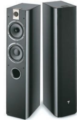
Chorus 716 is a 2.5-way loudspeaker with a high-end configuration thanks to its two 6.5" (16.5cm) speaker drivers working in tandem (only the top driver transmits the midrange). This configuration doubles the effect of the bass, perfect for rooms measuring up to 320ft<sup>2</sup> (30m<sup>2</sup>).
