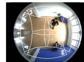
Four virtual PTZ cameras out of a single 360° hemispheric camera
