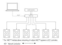
Using a network enabled VNET SC1 to combine an existing Tannoy VNET™ system with another loudspeaker system (e.g. Tannoy POWERV™)
