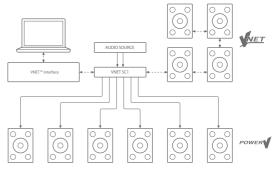
\* The VNET™ interface allows networking of multiple VNET™ speakers or SC1 controllers
