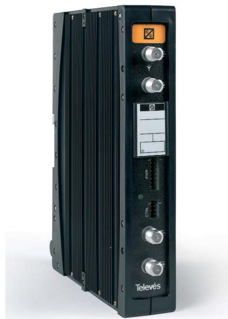
Analog & digital channel processor allowing the conversion or just processing of both digital & analog channels. Fully input/output agile through the full VHF & UHF band. The product can also be used as channel processor using same input/output channel. The input AGC guarantees a stable output level.
